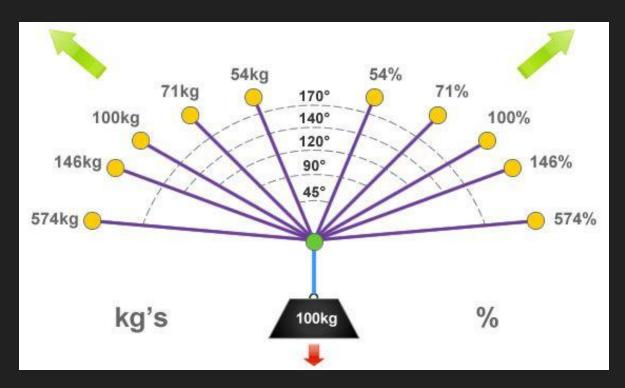
Before the first test jump, we used this vector force chart to estimate maximum possible forces. The canopies mirror and amplify each others force until pulling the system so taught it accelerates. With no way to gather data on the exact pitch of these canopies, we decided to compare a gross amount of force to all the components to prove reliability.
